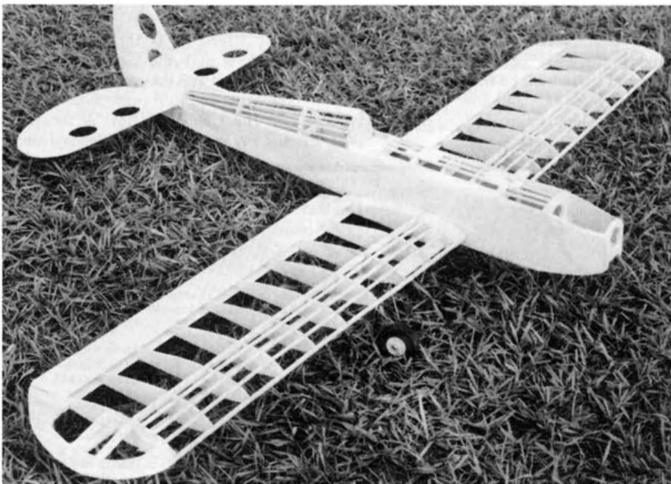
Bare bones ready for covering and equipment installation. Lightening holes in tail help keep the aft section light. When balancing the wing, remove weight from the heavy side.
