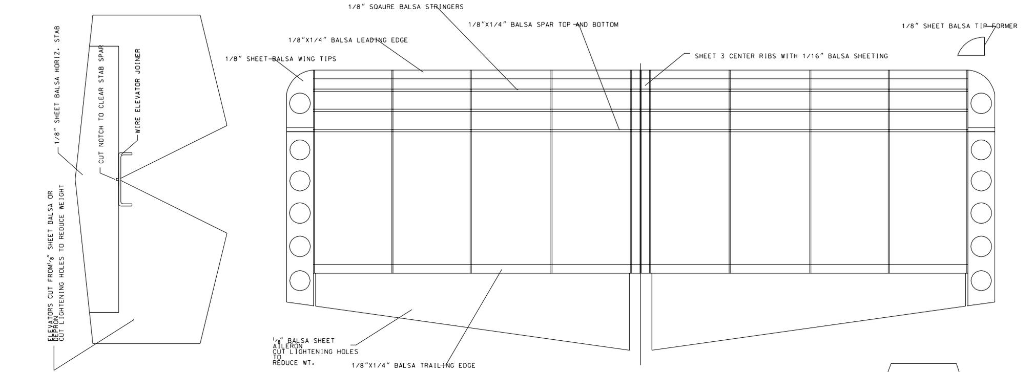
NOTE: CUT LIGHTENING HOLES IN RIBS TO REDUCE WT.
