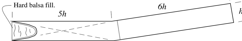
Cut back joiner's middle along diagonals on glued-in side. This greatly reduces bondline stress concentration at the end.
